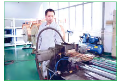
涨管 Copper Pipe Expanding
