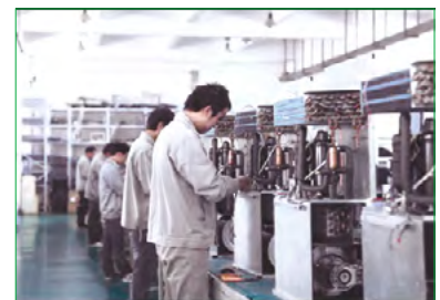
半成品检测 Half-Done Chiller Test
