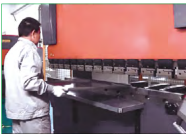
钣金 Chiller Frame Making
